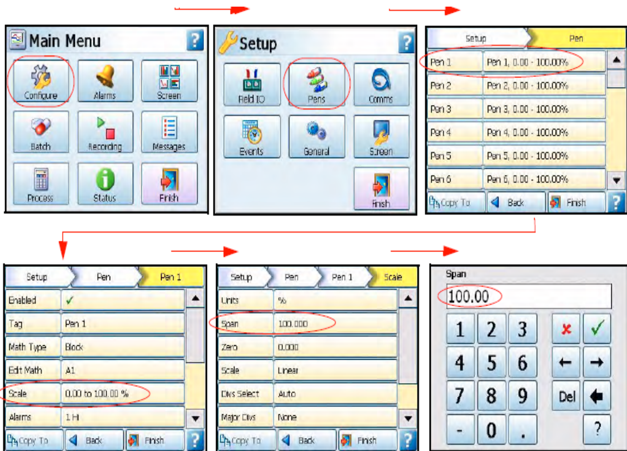
Example of a recorder menu path from the Main Menu to Pen Scale configuration with clear rapid navigation
